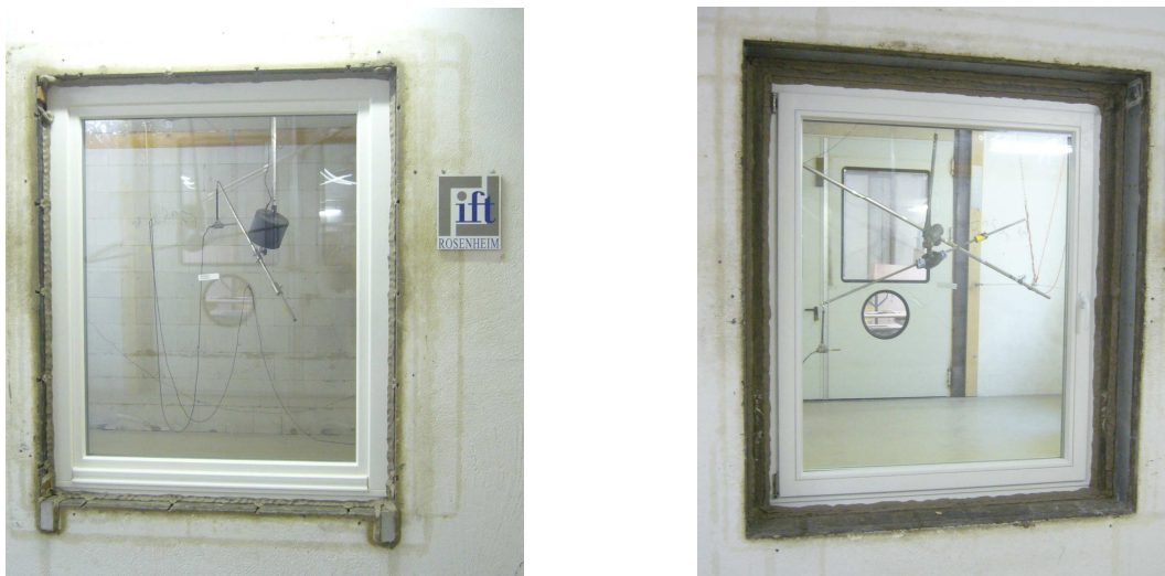
Fig 1 Photo(s) of the mounted element, taken by ift Laboratory for Building Acoustics
