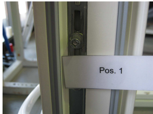
Fig. 8 Locking situation casement Pos.1
